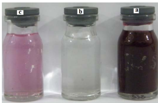
Figure 12. The photos of (a) feed solution, (b) permeation from PES/0.1 wt % goethite membrane (c) permeation from unfilled PES membrane. [Color figure can be viewed in the online issue, which is available at wileyonlinelibrary.com .]
